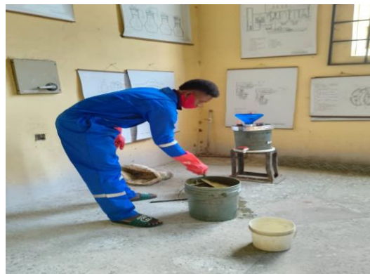
Plate 4: Feeding the digester with the formed slurry
